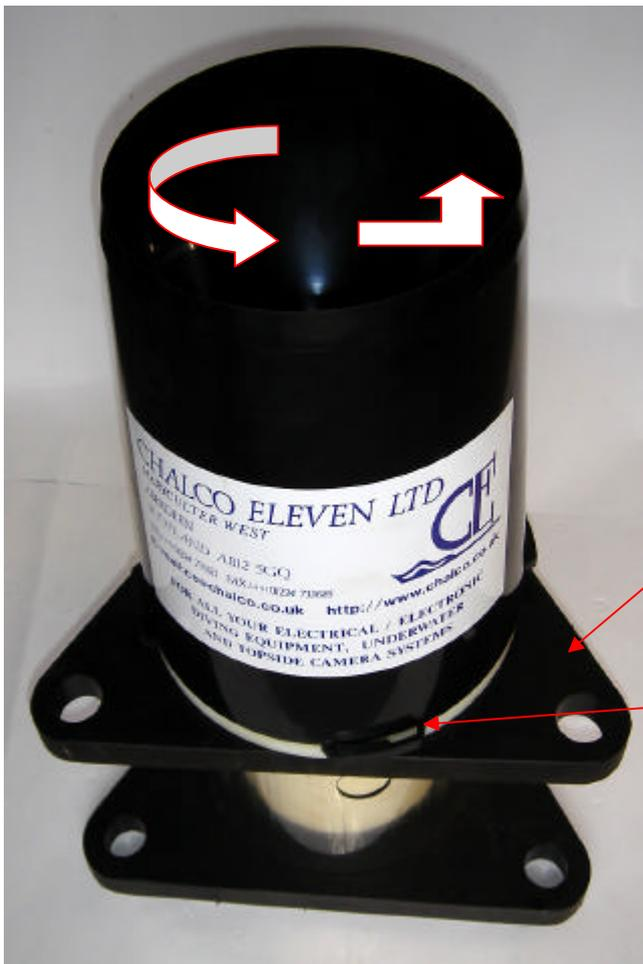
Twist the Bucket anti-clockwise 10 degrees holding the Middle Securing Flange until the slots line up. Then lift the Bucket up gently.
