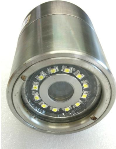
The CHB65MM is a high resolution Digital Colour Camera designed for underwater / Pipe Line Inspection use. The Camera has a depth rating of 300ft MSW and is designed for harsh and unpredictable low light environment. The CHB65MM is equipped with a specially developed circuitry by Chalco Eleven known as the electric eye and also incorporating high intensity SMD LED's for daylight illumination.
